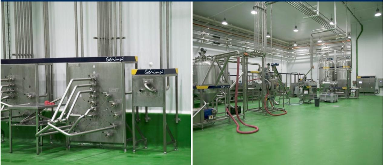
Pasteurization line with deaerator and storage in an aseptic tank prior to packaging.
