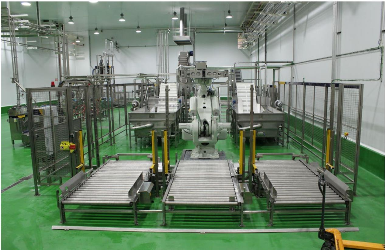
New development for the production of melons and watermelons: extraction of the pulp without mashing and mixing the outer rind, which produces an exquisite quality pure melon or watermelon cream ready to be refined and clean of seeds before the heat treatment previous to the aseptic packaging.
