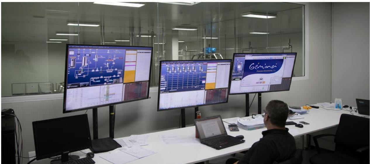
The process is completely automatic and integrated for controlling the production and registering the process data.
