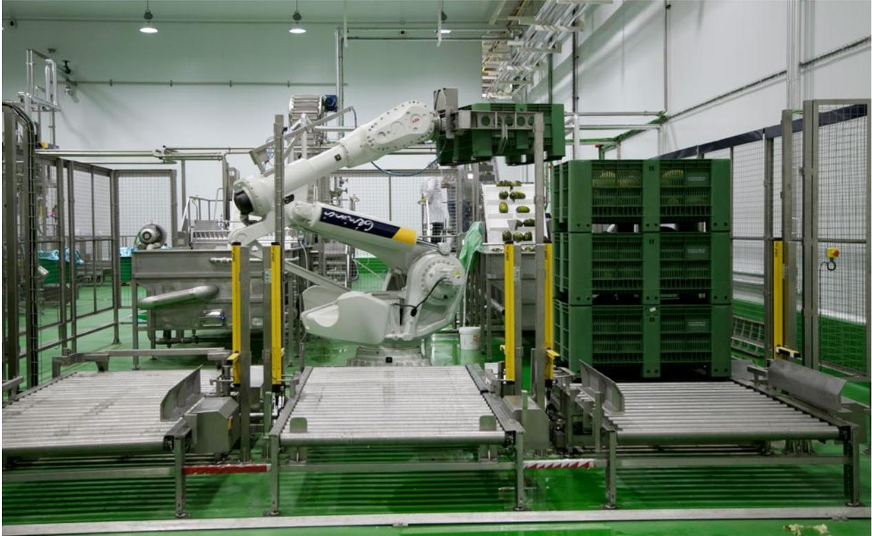
Line including thermophysics peeler for tomato peeling and its following grinding for packaging in tubs.
