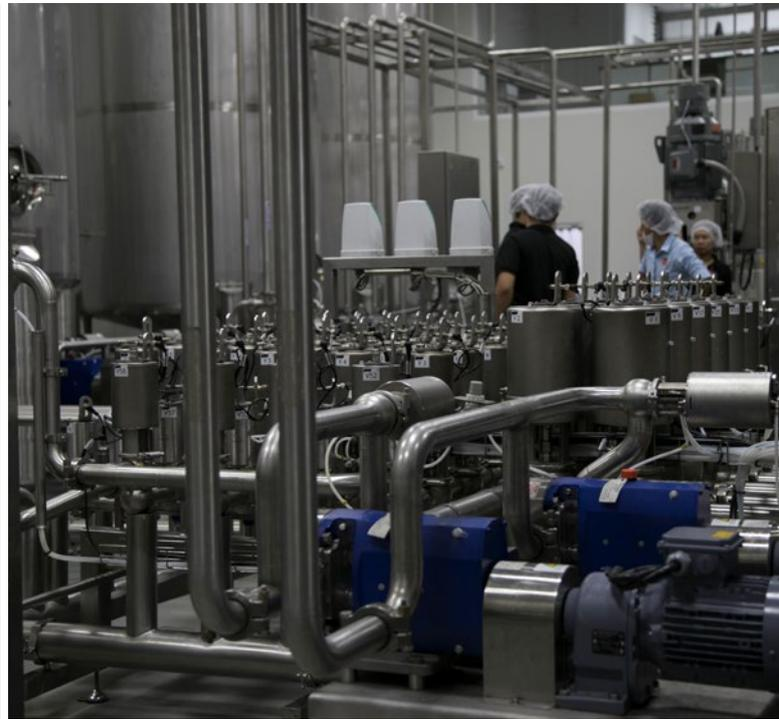
Automatic raw material room with preparation and recipe record for dosage of different ingredients such as chili, sugar, pieces of vegetables, garlic sauce... and combining a kitchen of 7 heated tanks with mixing for recipes preparation.
