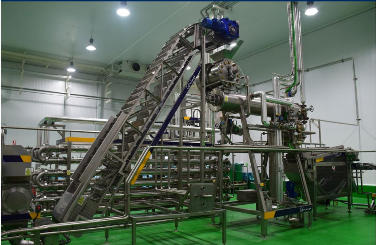
Grinder of hammers, extractors, sieves and finisher for different extraction treatments depending on the product.
