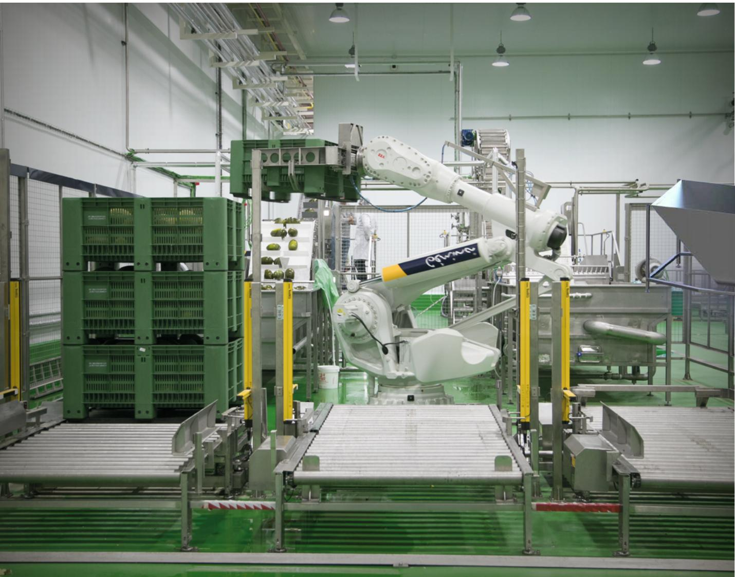
Anthropomorphic robots can be programmed to handle any element. Therefore, Gémina designs and creates solutions adapted to the different customer's needs. Gémina also creates different solutions for different containers: metallic or plastic drums, pallets, boxes, cans, bags, packs, etc.
